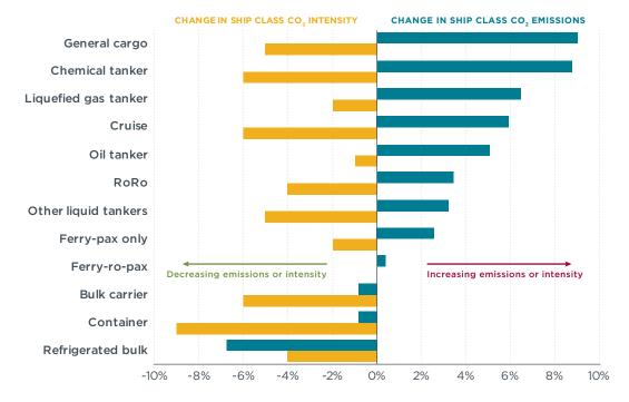
Figure ES-4. Change in CO<sub>2</sub> emissions and CO<sub>2</sub> intensity for key ship classes
