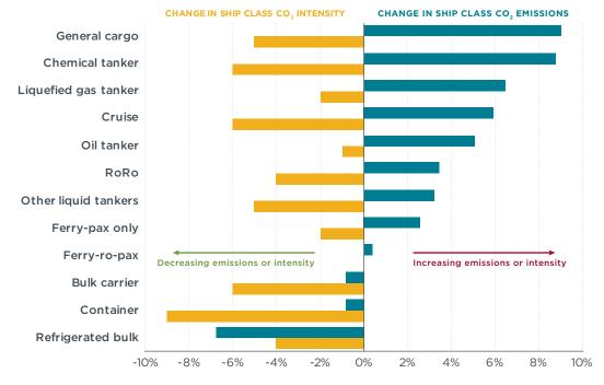
Figure 9. Change in CO<sub>2</sub> emissions and CO<sub>2</sub> intensity for key ship classes
