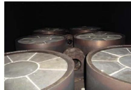
Particles can be efficiently removed by particulate filters.
